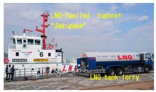
LNG-fuelled tugboat during LNG bunkering at the Port of Yokohama
